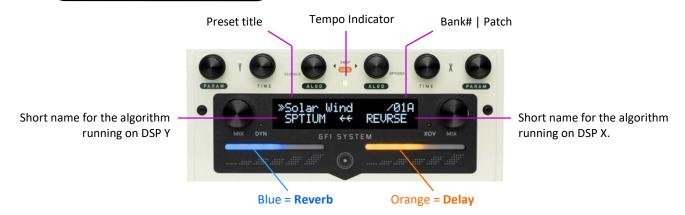
**Dynamics LED indicator** lights up when Dynamics X and(or) Dynamics Y are active.
