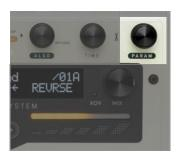
Each algorithm has 8 unique parameters. These parameters are controlled using a single knob, the PARAM knob.
